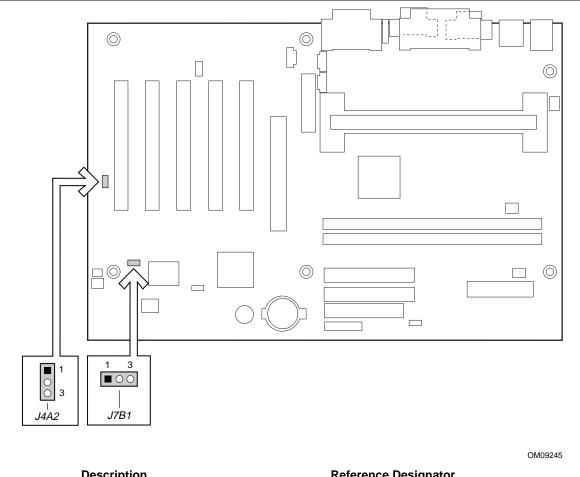
**Description Reference Designator** S5 remote control jumper block J4A2 BIOS setup configuration jumper block J7B1
